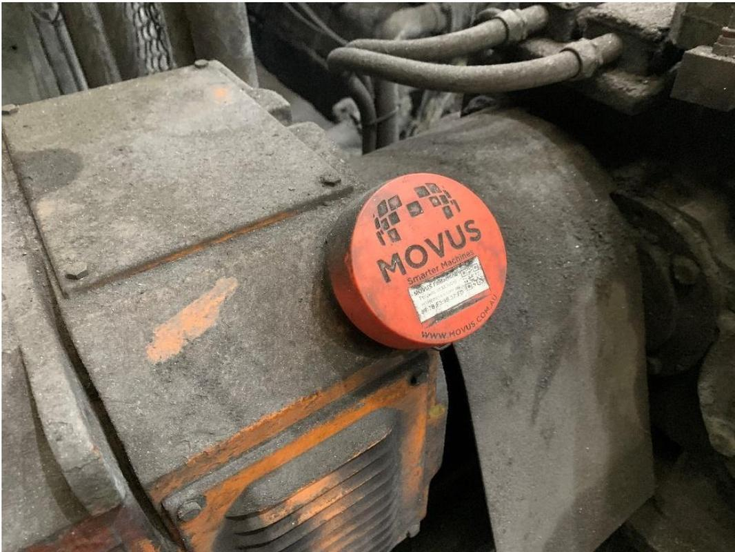
Figure 2. MOVUS FitMachine installed on equipment.
