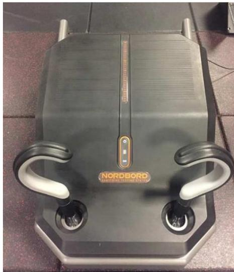
**Figure 2.** The NordBord measures approximately 3 feet by 2 feet, with much of its surface covered by a pad for athletes to kneel on. Positioning is easy, with athletes slipping their ankles into the padded, ergonomic ankle hooks.
